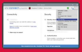
▲ Send files from Raspberry Pi using the File Transfer option in VNC Server in Raspbian. Use the three-bars menu (top-right) to find it.
